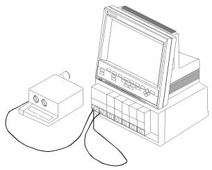
Agilent V24 Monitor with 15210B Calibration Unit
