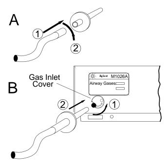
Attaching the Gas Sample Tube to the Module
